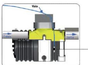
**PLAATSINGSSHEMA ALARM / SCHÉMA D'IMPLANTATION TYPE DE L'ALARME**
