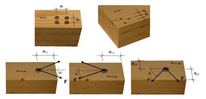
Definition of spacing, end and edge distances in the edge surface:
