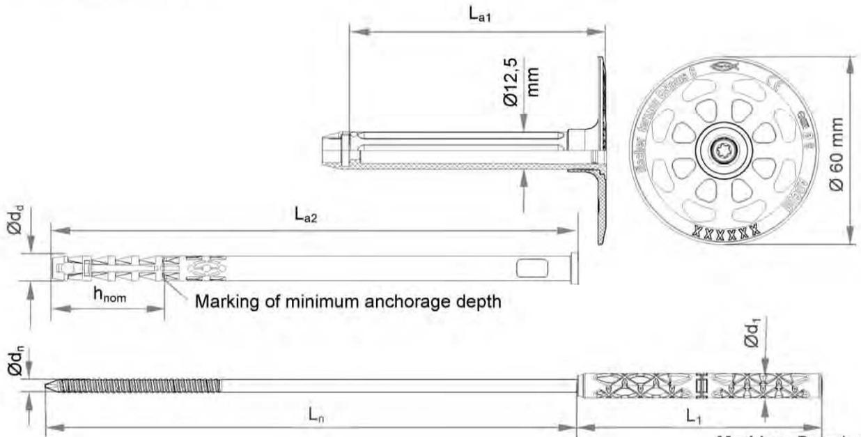
**Marking:** Brand, name and size of anchor, diameter, categories, optional markings see drawing of anchor plate, example e.g. termoz CNplus 8 ABCDE
