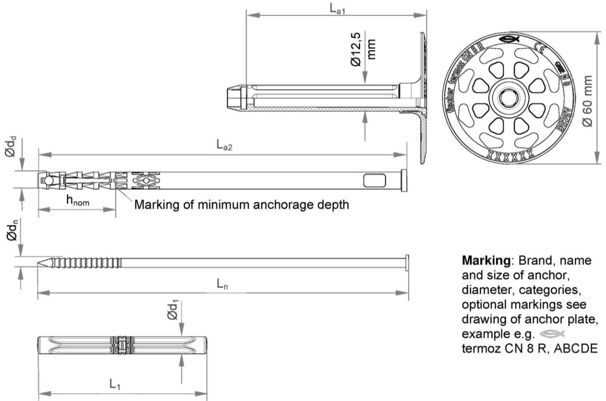
**Marking:** Brand, name and size of anchor, diameter, categories, optional markings see drawing of anchor plate, example e.g. termoz CN 8 R, ABCDE
