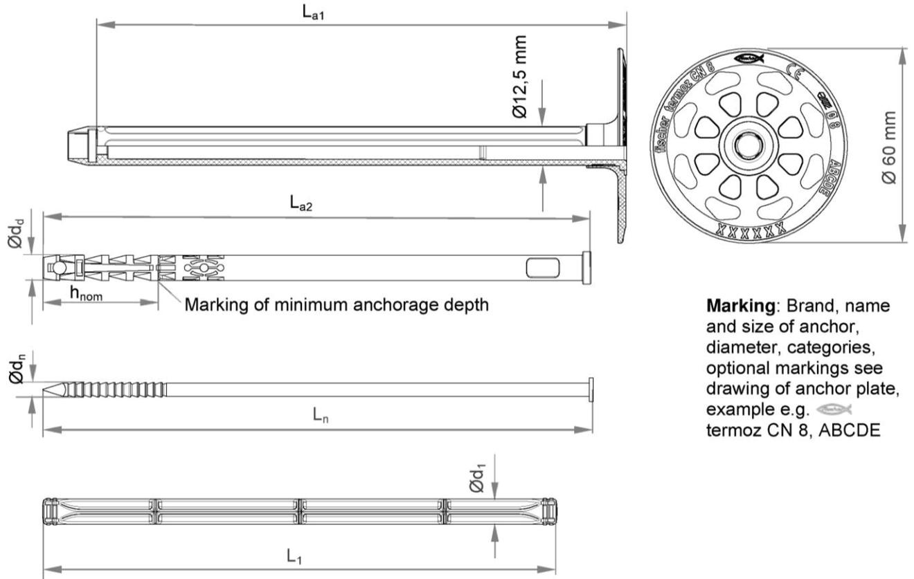
**Marking:** Brand, name and size of anchor, diameter, categories, optional markings see drawing of anchor plate, example e.g.
