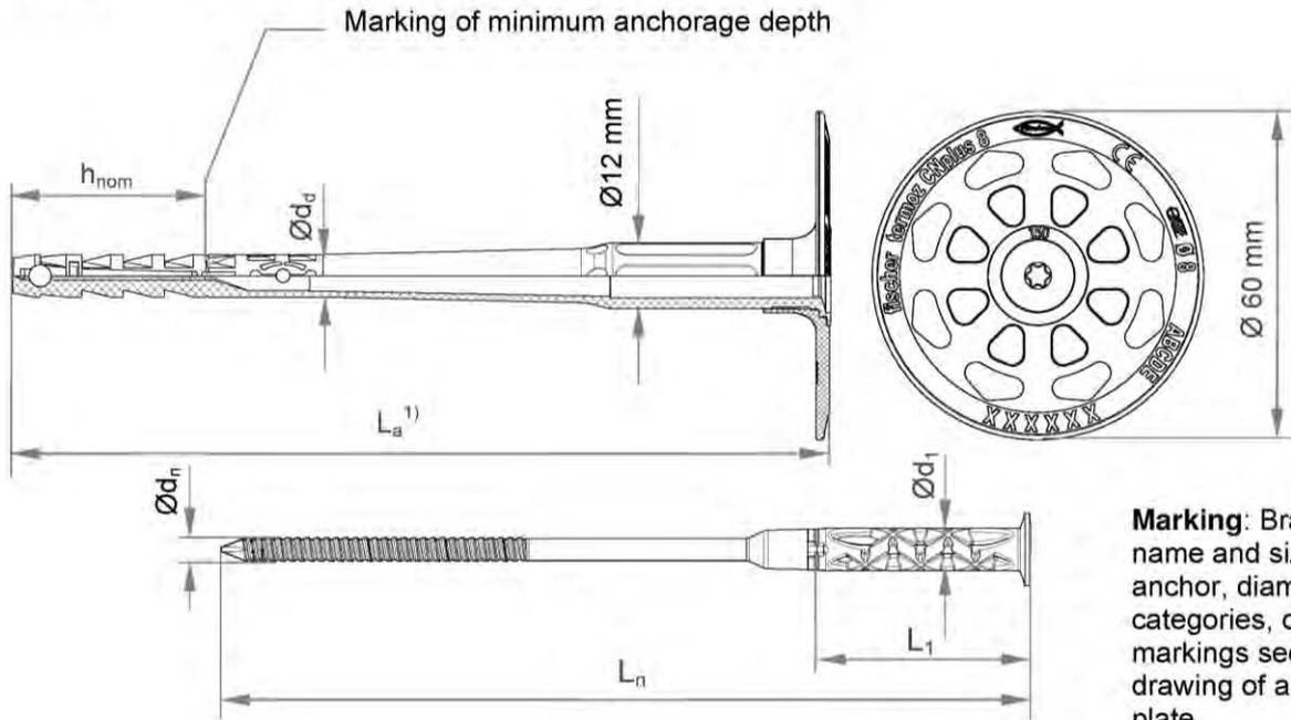
**Marking:** Brand, name and size of anchor, diameter, categories, optional markings see drawing of anchor plate, example e.g. termoz CNplus 8
