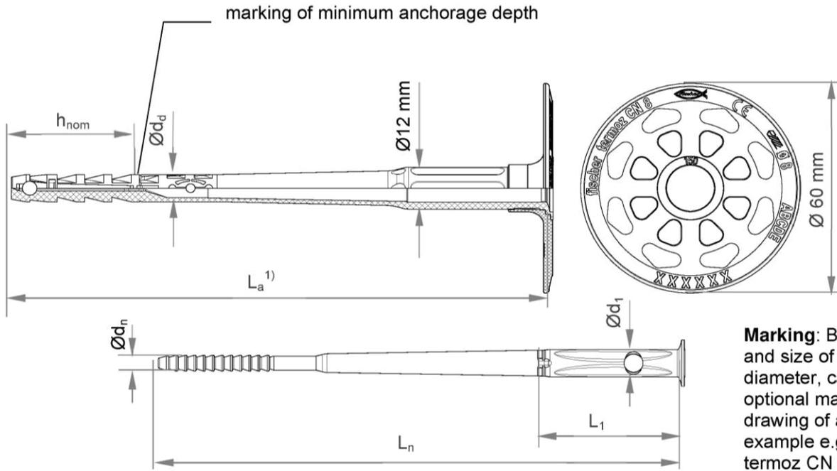
**Marking:** Brand, name and size of anchor, diameter, categories, optional markings see drawing of anchor plate, example e.g.
